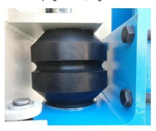
6, High elastic rubber ball, automatic screen cleaning, and avoid screen blocking.
