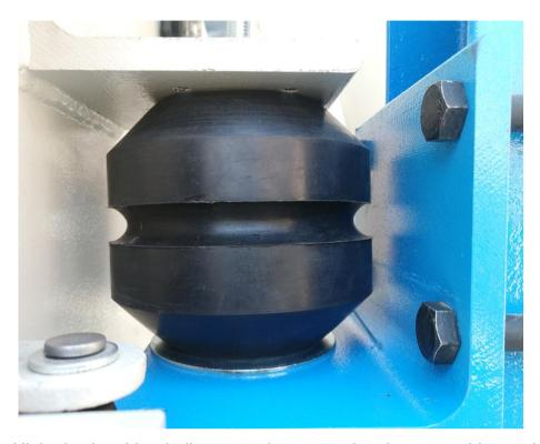
5,High elastic rubber ball, automatic screen cleaning, to avoid material particles blocking.
